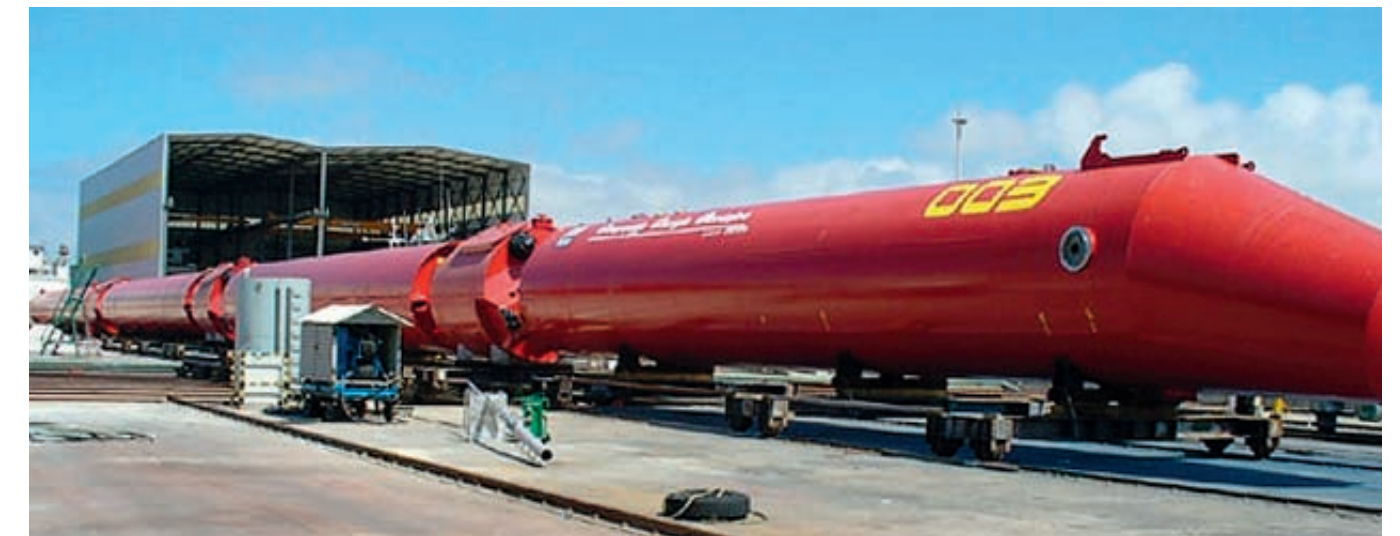
Figure 335 Pelamis wave energy converter Length approx. 150 meters, diameter 3.5 meters, weight including ballast 700 tons Source: Pelamis Wave Power Edinburgh, Scotland. UK
